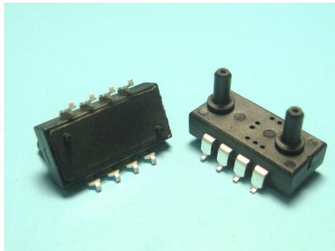
The MIS-3610 is an intelligent pressure sensor which consists of a MEMS piezoresistive pressure sensor and a CMOS sensor interface IC. The interface IC enables easy and precise calibration of resistive bridge sensors via EEPROM. It corrects digitally offset, gain and both temperature coefficients. All devices were factory calibrated and temperature compensated. The MIS-3610 can provide 3V or 5V rail-to-rail ratiometric analog output.
